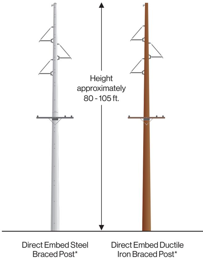
\*Final structure height, structure type, and ROW easement width may vary.
